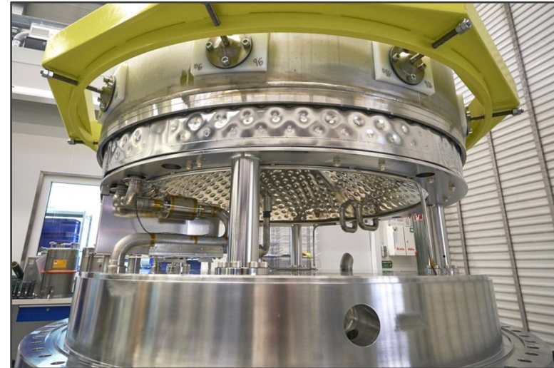
Figure 2. Photograph of ITER cryopump. Source: ITER.org.
